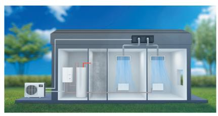
**PXZ for summer** PXZ enables cooling of multiple rooms by ATA and supply hot water by ATW.
